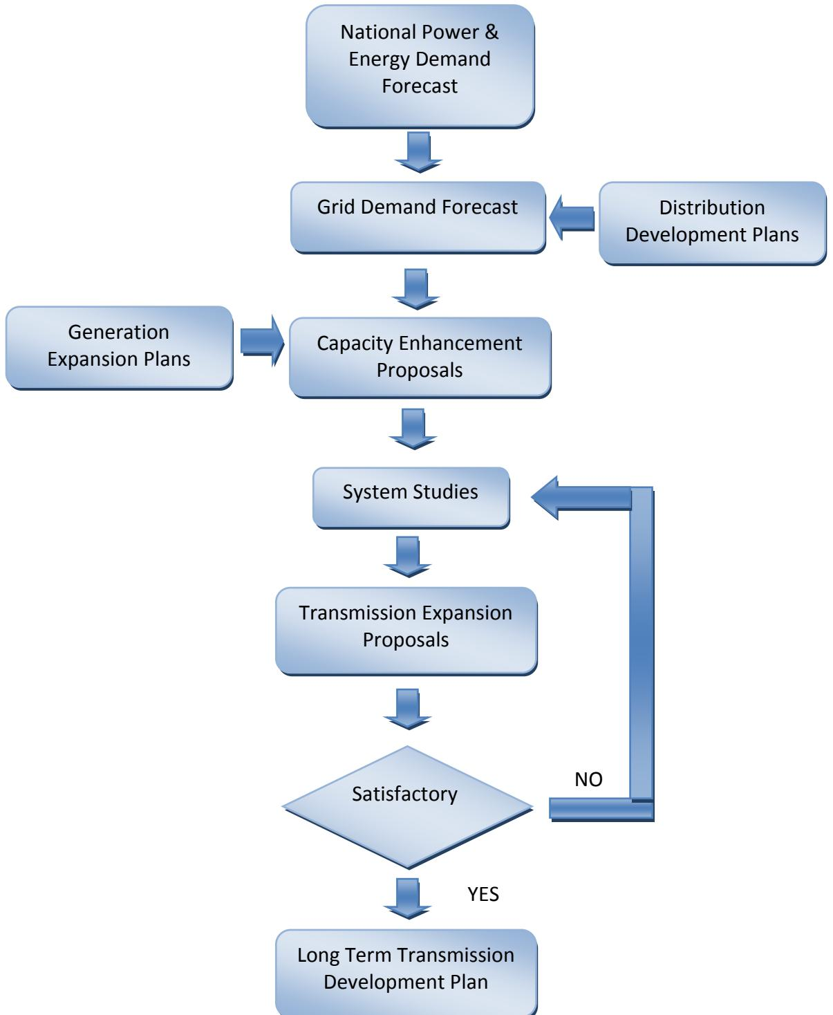
**Figure 2: 1 Schematic representation of the transmission planning process**
