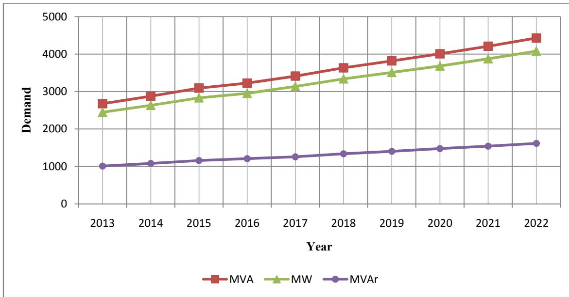
**Figure 3.1: Grid substation demand variation at system peak**
