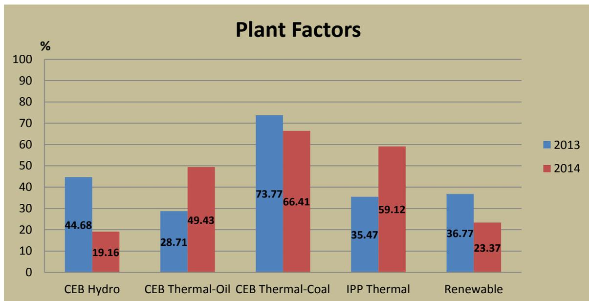
Overall plant factors of CEB hydro plants and Renewable plants have been dropped down due to low rainfall, which has highly impacted towards increasing of thermal oil plant dispatch.
