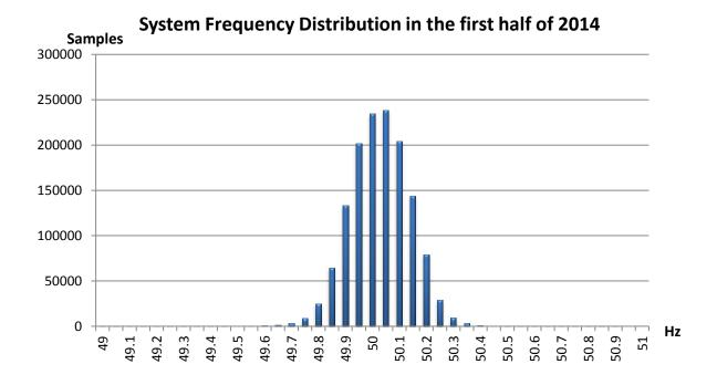
To figure out the extent of frequency excursions, three frequency ranges can be defined as follows
