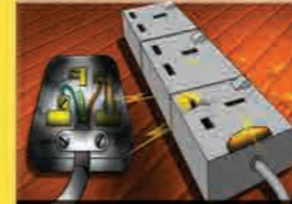
Burn marks on plugs, leads or appliances
