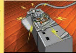
Cracked or damaged cases on plugs & appliances
