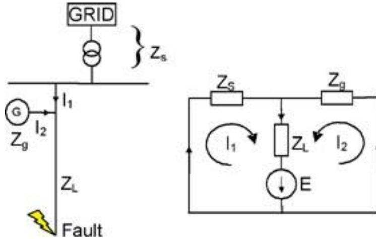
The impact of this phenomena increase with the size of DG unit as it would contribute more to the fault current. Furthermore, the fault current generated from DG in short circuit faults, strongly depends on both generator type and network configuration. Synchronous generators can feed rather large and sustained currents while inverter based systems in most cases, will be controlled so that their output is limited to rated current.
